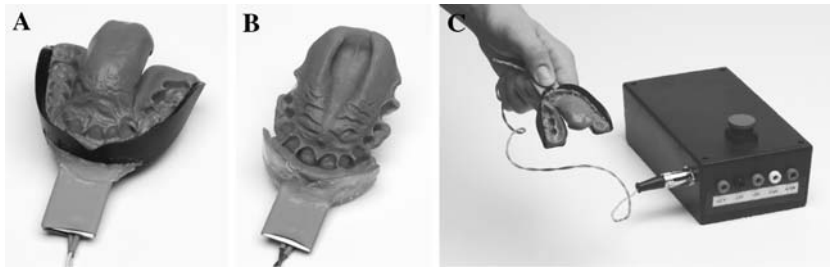
Fig. 2. (A) MOST I and (B) MOST II mouthpieces are shown, along with the (C) MOST I mouthpiece and electrical circuit.
